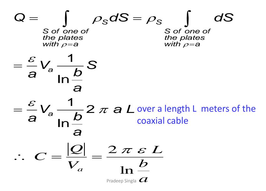
Therefore the capacitance per unit length of the line  $C_L$  is
